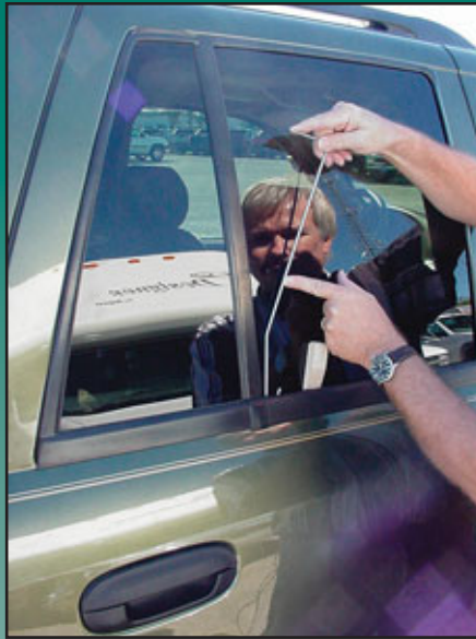
5. Insert the TT-1001 tool with the hook pointed forward.
